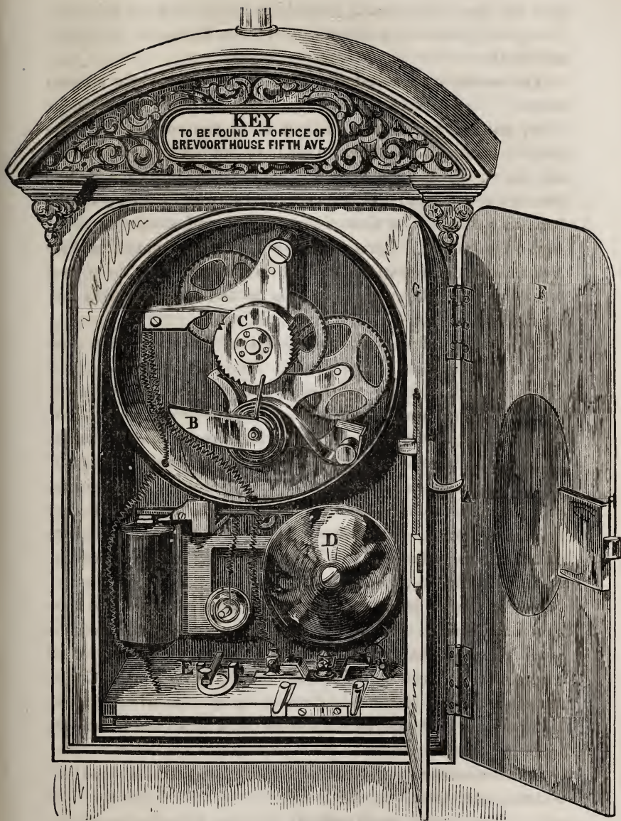
FIRE ALARM SIGNAL-BOX.
